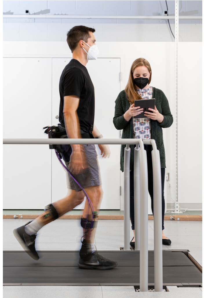
Clinical scientist Alyssa Spomer evaluates real-time feedback from the Biomotum SPARK ankle exoskeleton, which can assist and resist ankle motion to support gait training and rehabilitation.
