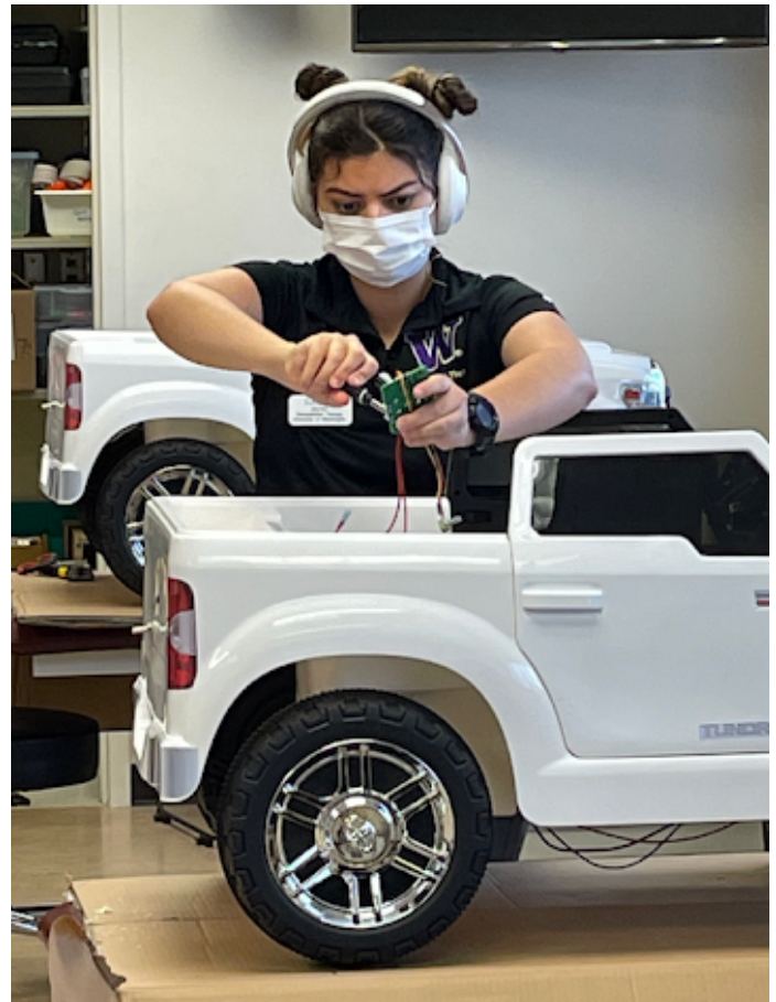
A Go Baby Go workshop volunteer connects a speed controller that will enable kids and families to adjust speeds while driving their custom modified ride-on car.
