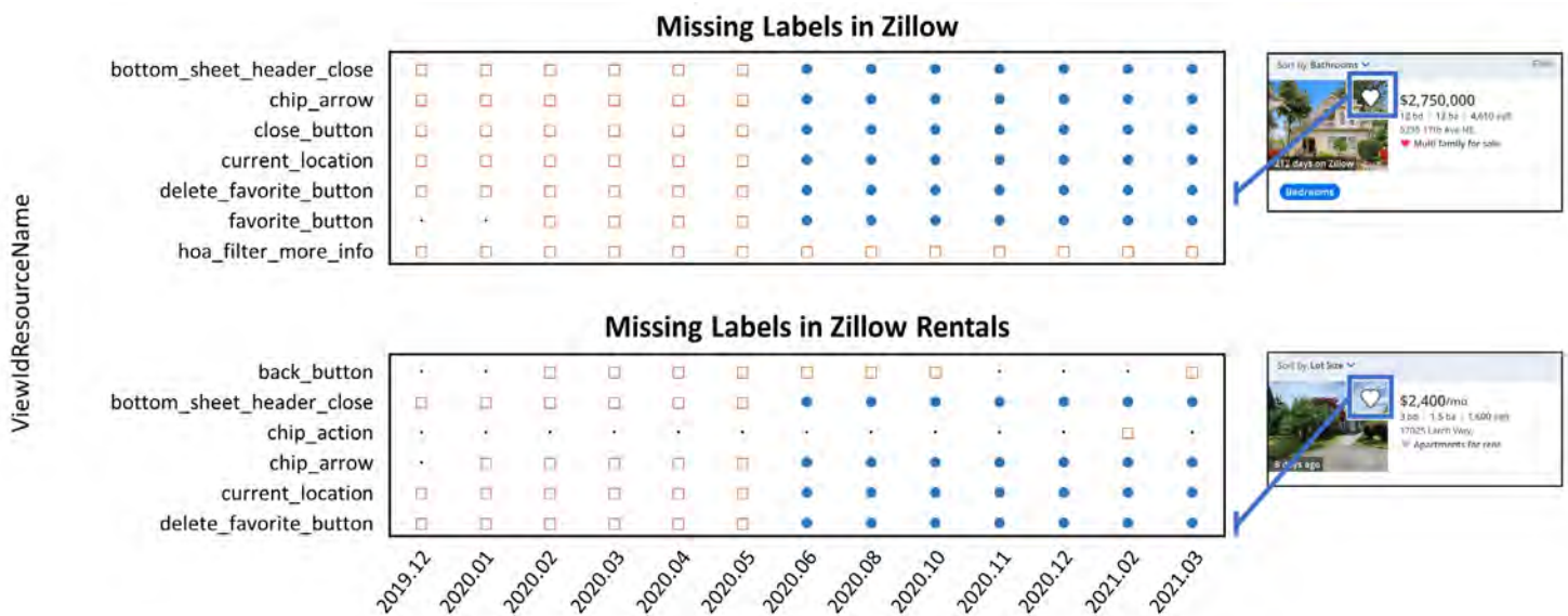
Above are two failure plots enabled by our unique longitudinal dataset, each visualizing a 16-month period of missing label failures in applications published by Zillow: a home-buying application (top), and an apartment rental application (bottom). An empty orange square indicates a unique element observed to have a missing label failure, a solid blue circle indicates a unique element observed as labeled, and a black point indicates the element was not observed in that snapshot. The June 2020 snapshot clearly shows repairs to longstanding missing label accessibility failures. The two applications also share four ViewIdResourceName values, suggesting these repairs may have been the result of a systematic accessibility improvement in shared code.
